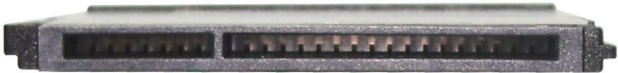
Figure 4: SATA 7-pin (data) + 17-pin (power)
