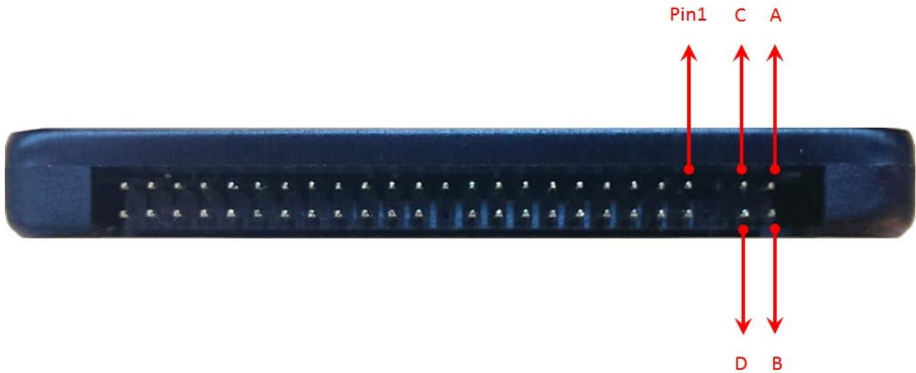
Figure 3 : The connectors of 2.5" PATA MLC SSD
