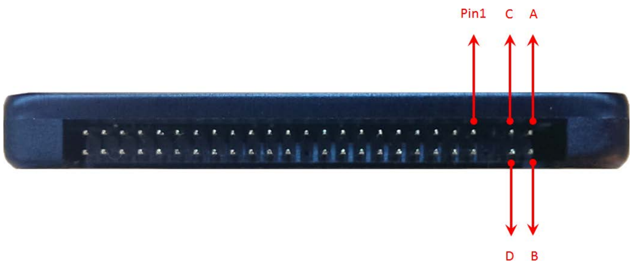
Figure 3 : The connectors of 2.5" PATA SLC SSD
