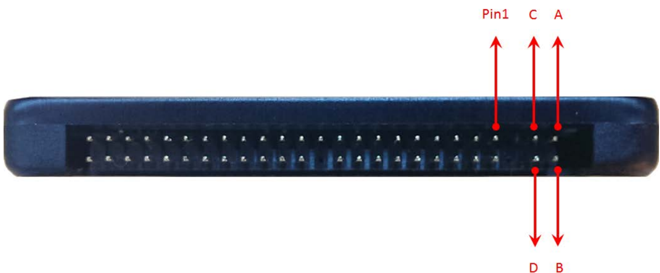
Figure 3 : The connectors of 2.5" PATA SLC SSD
