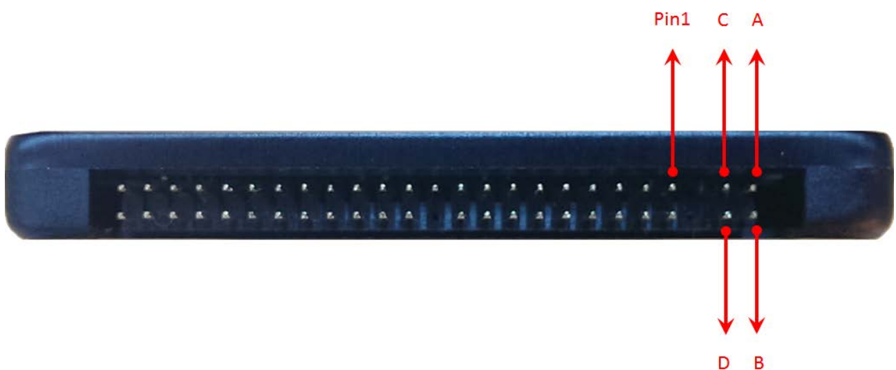
Figure 3 : The connectors of 2.5" PATA SLC SSD
