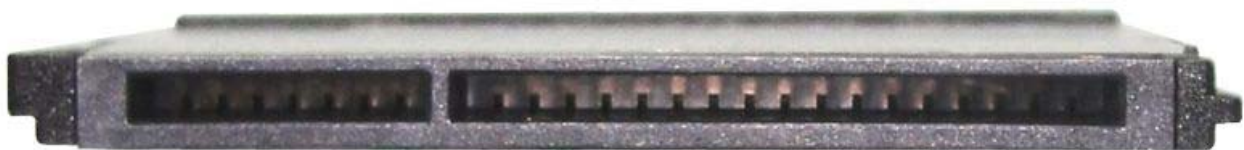
Figure 4: SATA 7-pin (data) + 17-pin (power)
